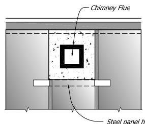
Steel panel hanger recessed into the top of panels. Typically 80 x 8mm corrosion protected MS, or similar, as sized by the project engineer
