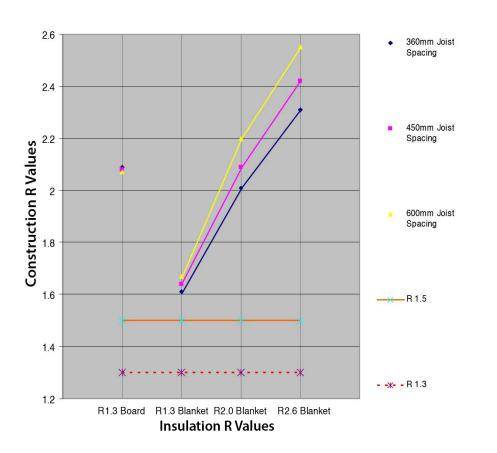
1. For open/exposed subfloors. Add the R Values for ground under a suspended floor (see separate sheet) to the above figures
